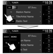
The unit is in standby to switch to Traffic Information (TI) if available. (The TI indicator lights up in white.)
