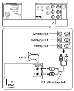
\* When connecting to an external amplifier, connect its ground wire to the car's chassis.
