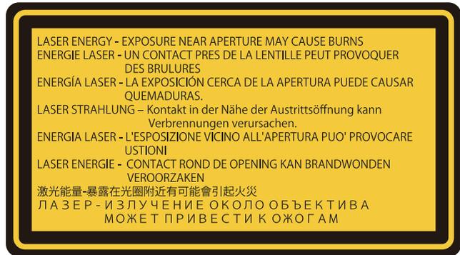
**WARNING: LASER ENERGY - EXPOSURE NEAR APERTURE MAY CAUSE BURNS
