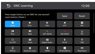
Touch a function button on the screen, then press target button on car SWC for more than 1 second.
