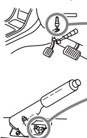
Parking brake switch (inside the car)
