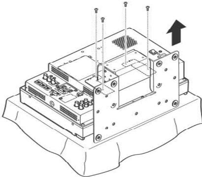
Using the mounting holes in the figure, fix the support plate with screws.
