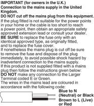
If these colours do not correspond with the terminal identifications of your plug, connect as follows: Blue wire to terminal coded N (Neutral) or coloured black.
